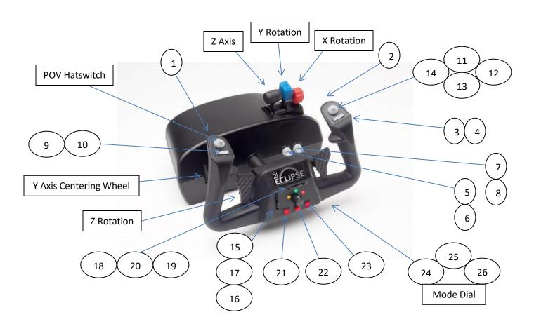
X Axis = Yoke Handle Turning Left and Right. In FS2020, assign "Ailerons Axis" to "Joystick L-Axis X"
